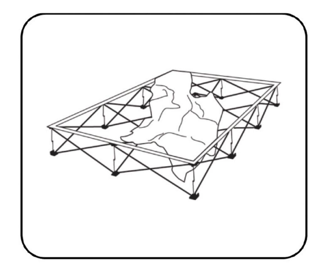
6. Attach the rest of the graphic by working your way around the frame. Make sure graphic is pulled taut while attaching the velcro.
